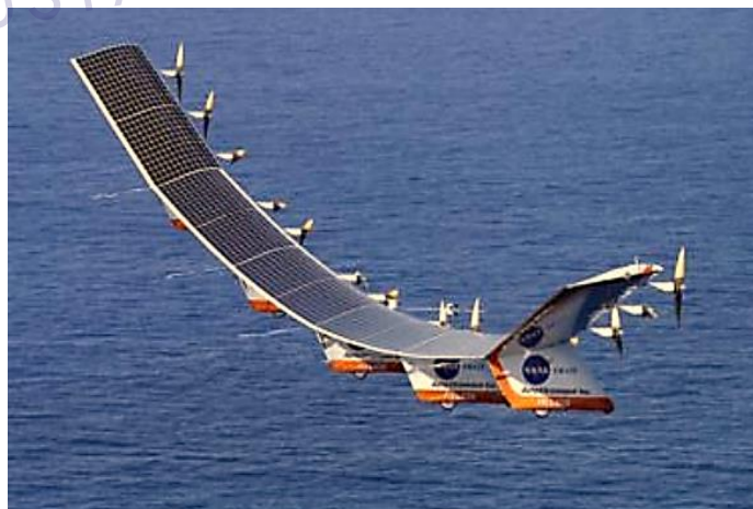
Figure 1.3: "Helios" solar powered UAV, developed by NASA [7]
