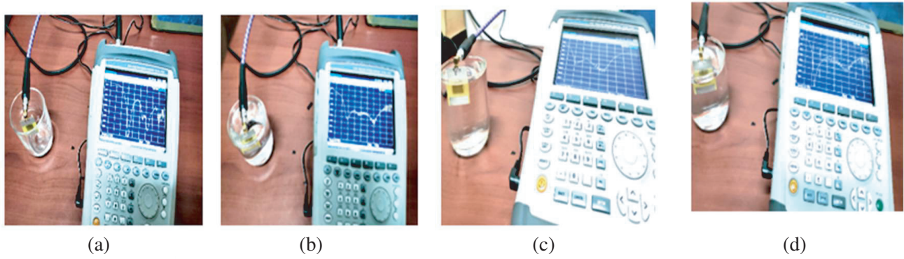
Figure 7. Different water solutions were tested by using a network analyser. (a) Air medium. (b) Distilled water. (c) RO water. (d) Raw water.
