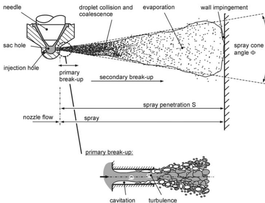
Figure 2.3: Relevant processes of a fuel spray [61].
