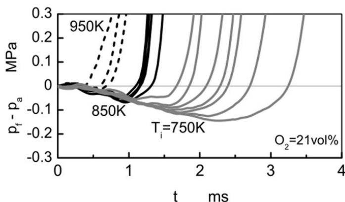
Figure 2.7: Histories of pressures during ignition delay period [79].
