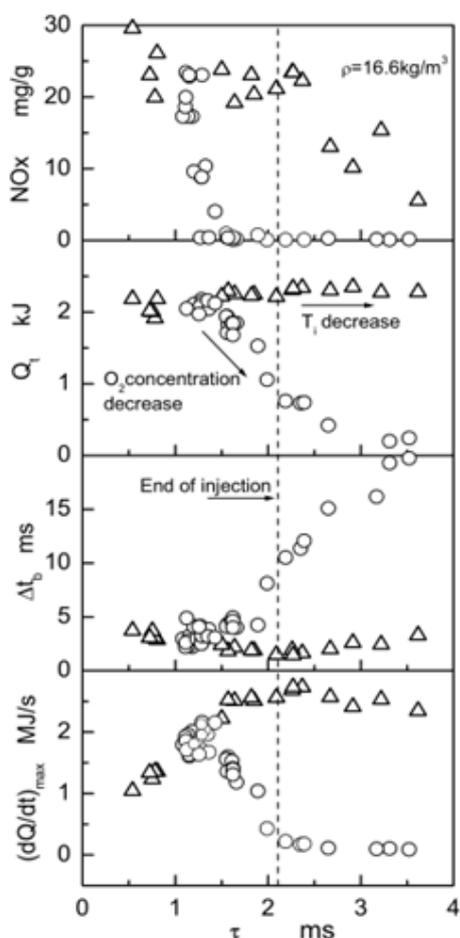
Figure 2.8: Relation between ignition delay and combustion characteristics [79].
