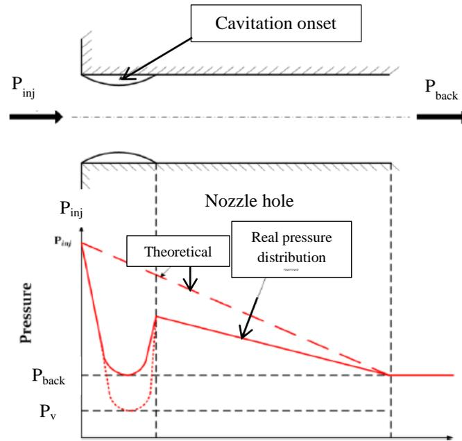
Figure 2.1: Cavitation formation inside nozzle [40]
