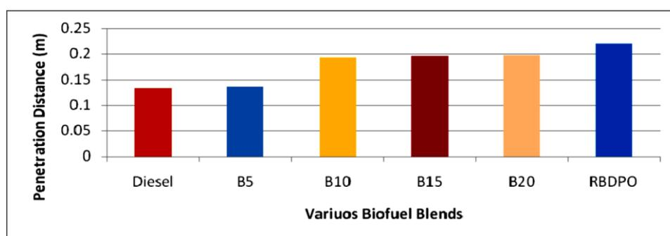
Figure 2.4: The graph of penetration distance (m) against various biofuel blends [70].
