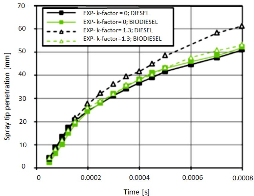
Figure 2.5: The graph of spray tip penetration against time [71].
