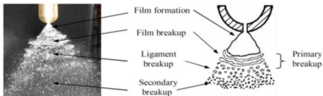
Figure 2.6: A typical spray pattern from spray nozzle [72].
