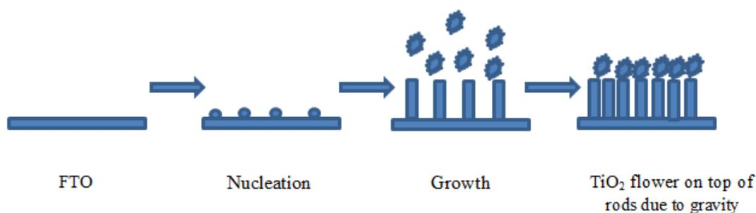
Figure 2.5: The growth mechanism of rutile phased  $\text{TiO}_2$  by hydrothermal method
