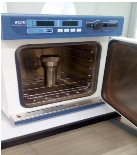
Figure 2.4: Autoclave for hydrothermal system in the oven
