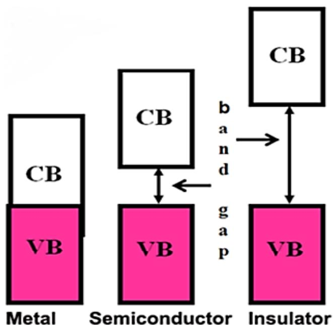
Figure 2.2: Valence band and conduction band for metal, semiconductor and insulator [21]
