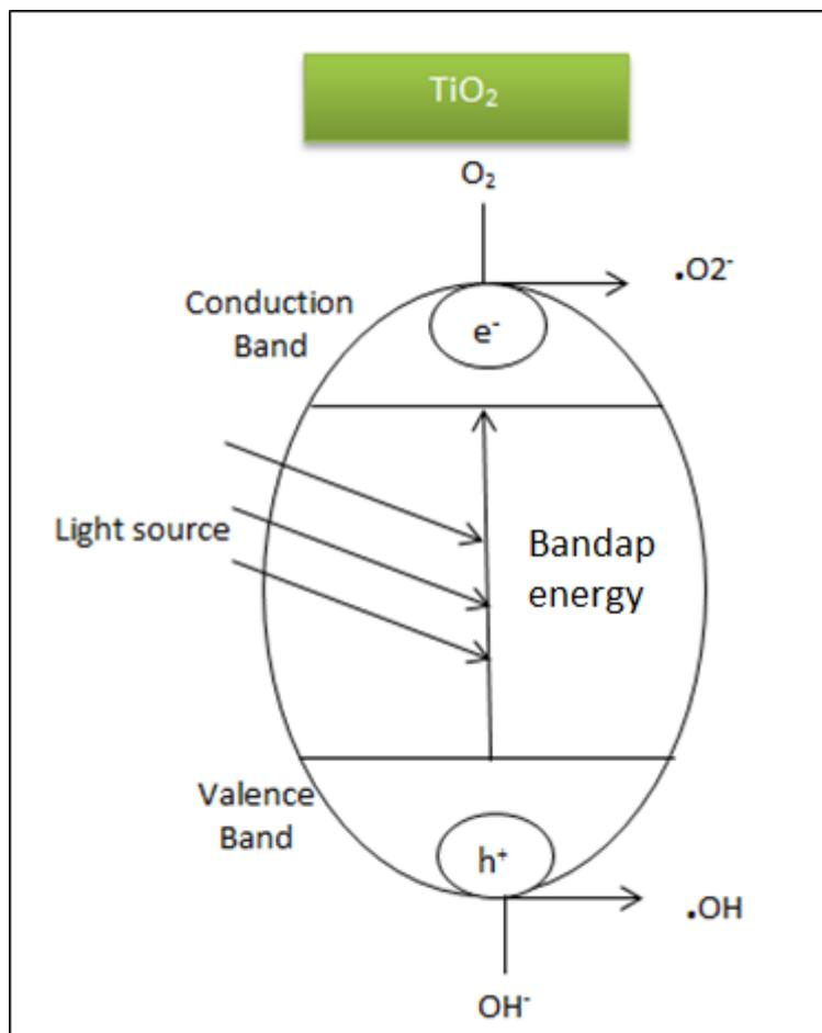
Figure 2.6: The mechanism of photocatalytic activity of  $\text{TiO}_2$  (reproduce image)
