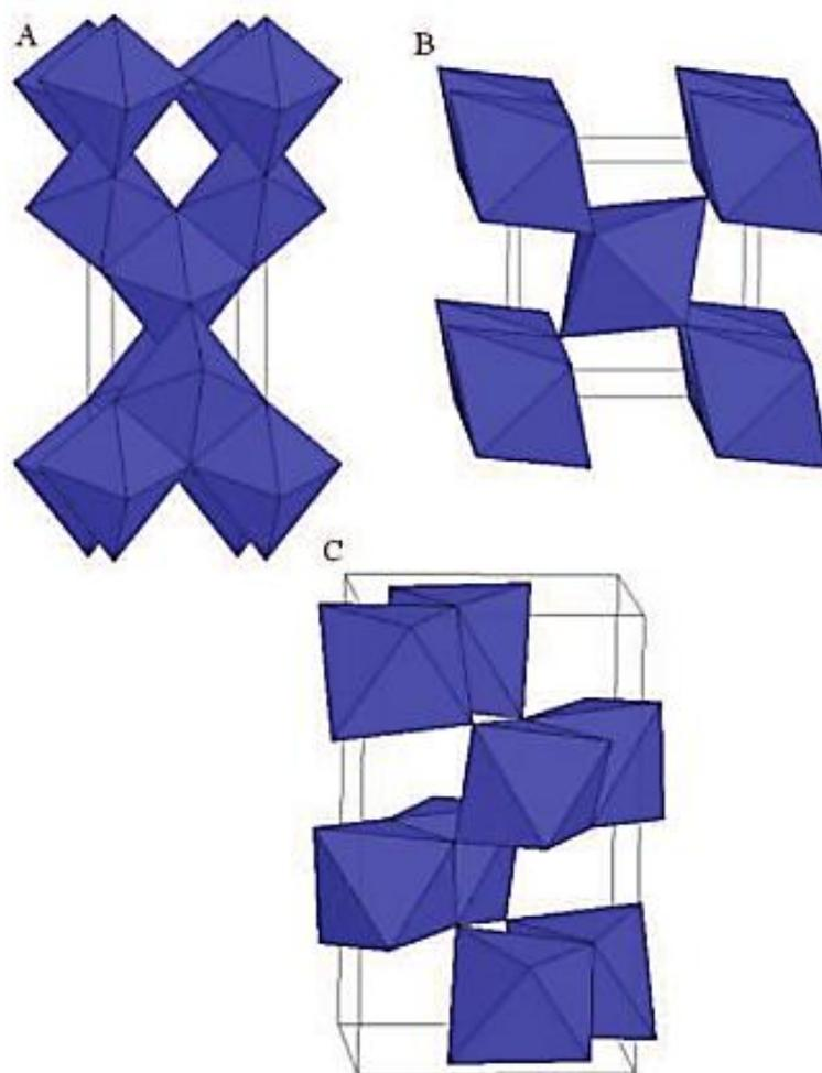
Figure 2.1: Crystal structure of (A) Anatase (B) Rutile (c) Brookite [20]
