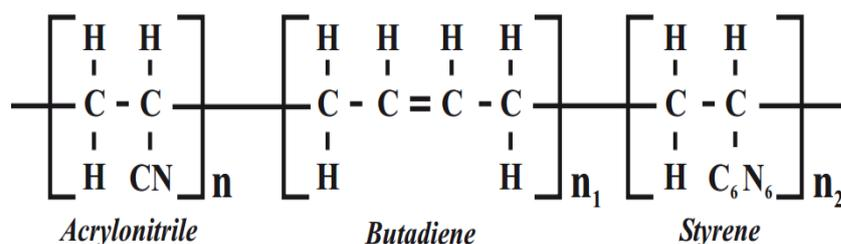
**Figure 2.9:** Chemical structure of ABS polymer (Wilks, 2001)
