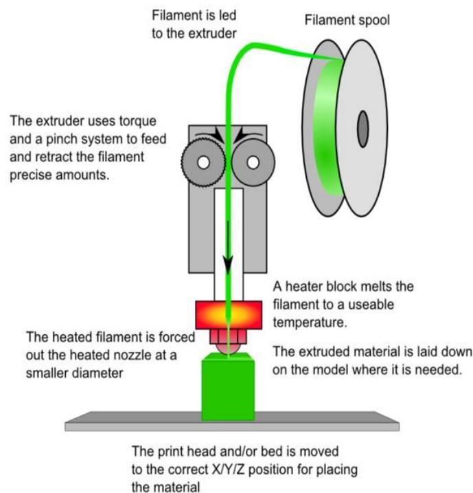
**Figure 2.8:** Schematic of Fused Filament Fabrication (3D PRINTING, 2014)
