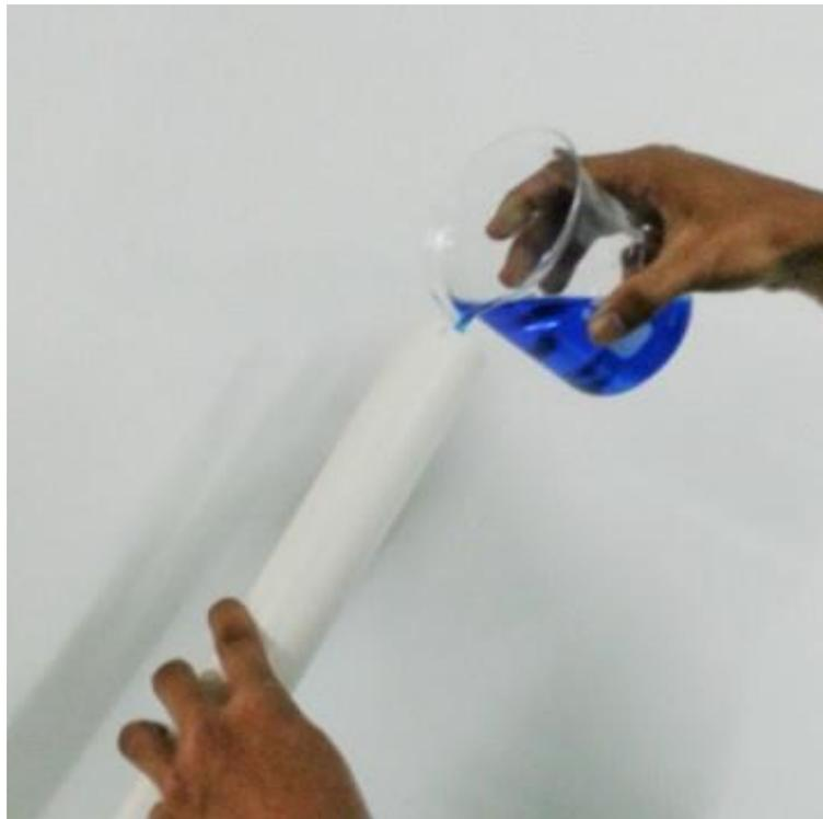
Figure 3: Method of pouring the liquid soap into the plastic mold
