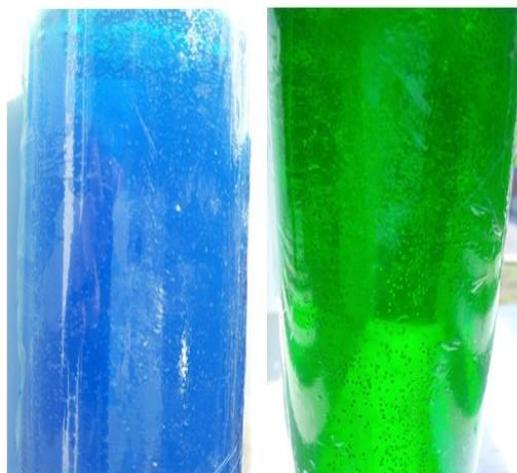
Figure 1: Tiny air bubble observed inside the soap
