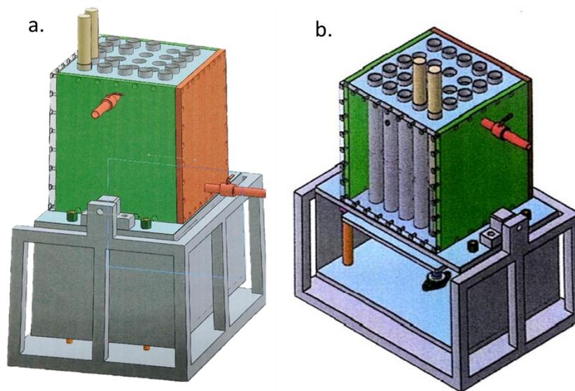
Figure 5: Diagram of the soap molder machine; a. Isometric View b. Sectioning View
