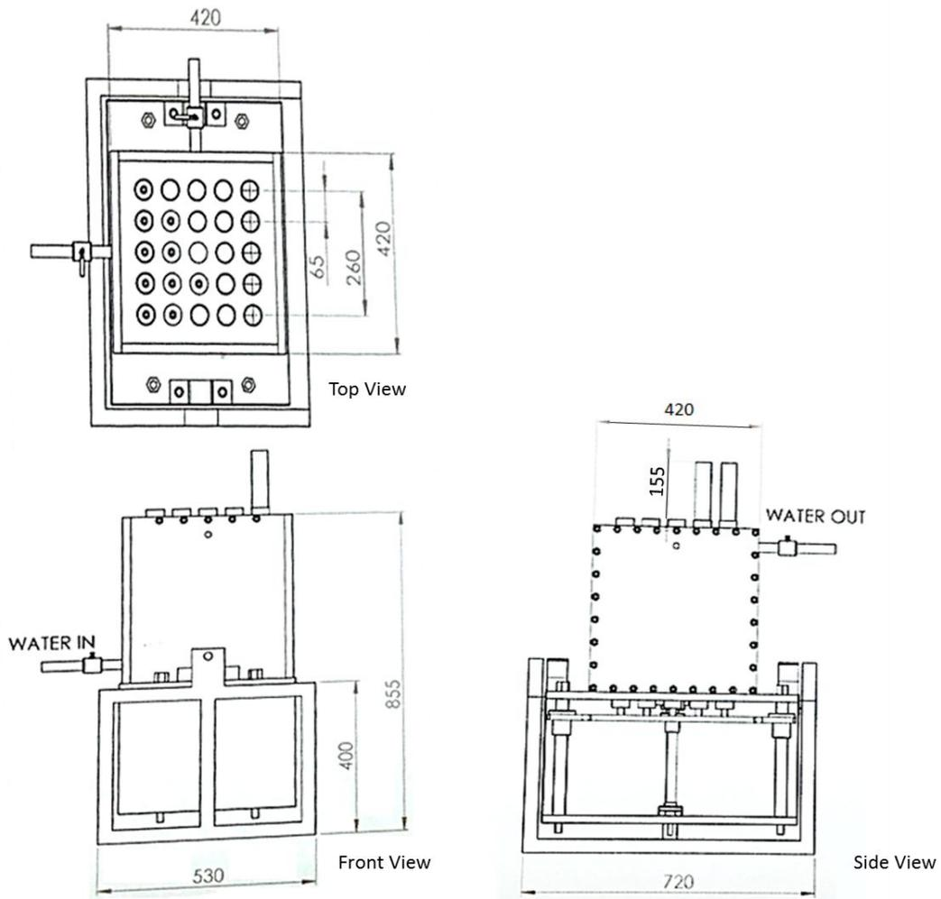
Figure 4: Layout diagram of the soap molder machine
