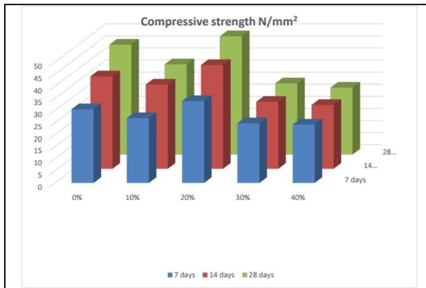
Fig. 5: Result of compressive strength for 7, 14 and 28 days [17].
