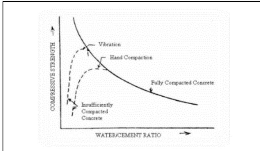
Fig. 1: The relationship between the strength of concrete and water-cement ratio [2]
