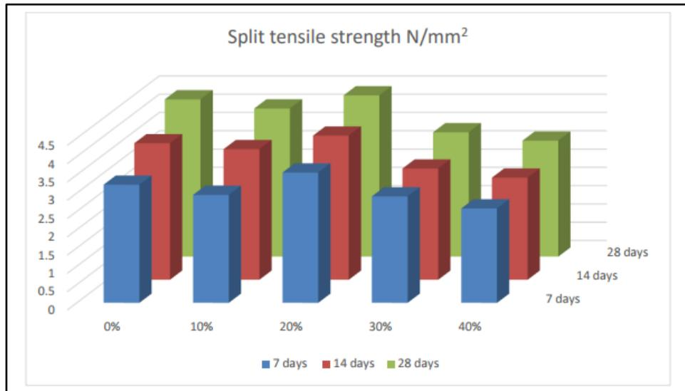
Fig. 5.2: Result of tensile strength for 7, 14 and 28 days [17].
