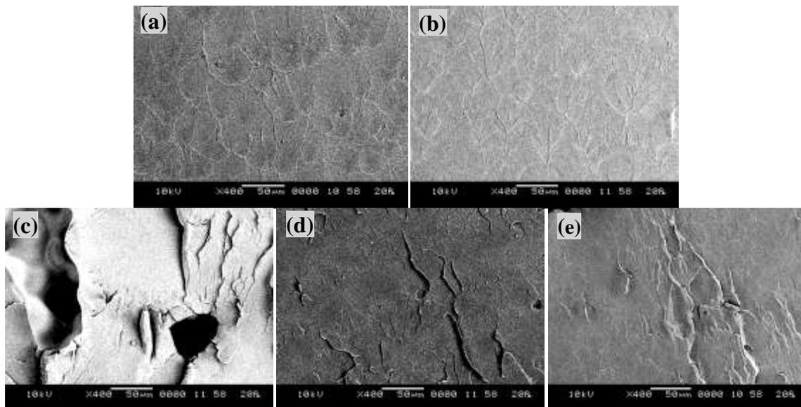
Figure 2: SEM of fracture specimen (x 400 magnification). a. Conventional technique; heat cure resin (Impact rapid repair material), b. Conventional technique; cold cure (impact rapid repair material), c. vacuum casting technique; no degassing (cold cure, Vertex Castavaria), d. vacuum casting technique; 20 sec degassing ( cold cure, Vertex Castavaria), e. vacuum casting technique; 40 sec degassing ( cold cure, Vertex Castavaria)
