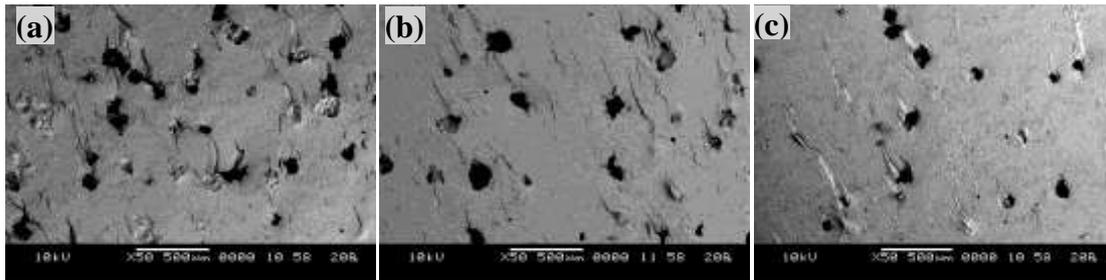
Figure 2: SEM (x 100 magnification) fracture specimen of cold cure (Vertex Castavaria) in vacuum casting technique, a. no degassing, (b) 20 sec degassing, (c) 40 sec degassing
