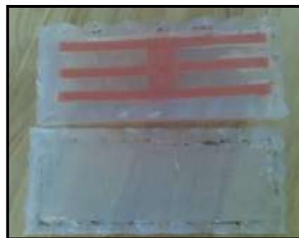
Figure 1b. Self cure resin (Vertex Castavaria) in silicone mould.
