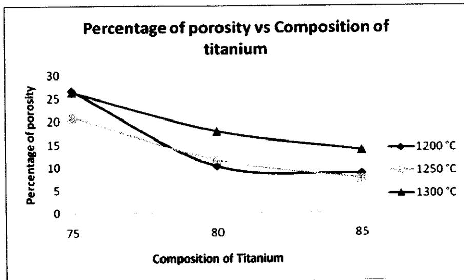
Figure 4: The effect of pure titanium foam content and sintering temperature on the percentage of porosity for the titanium foams
