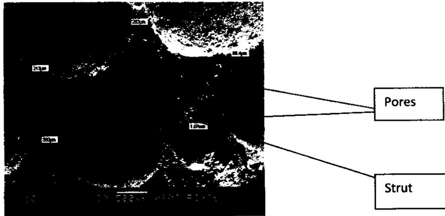
Figure 3: SEM micrographs of pure Titanium foam sintered in the tube furnace. The magnification for the sample is 30X
