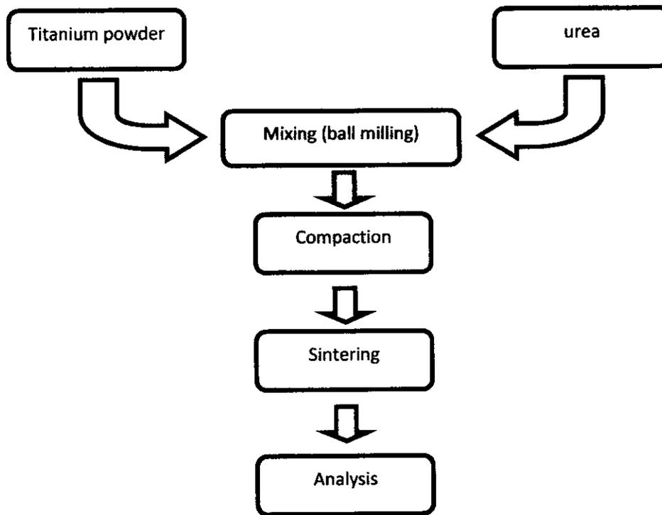
**Figure 2:** The flow chart for the sample preparation of titanium foam
