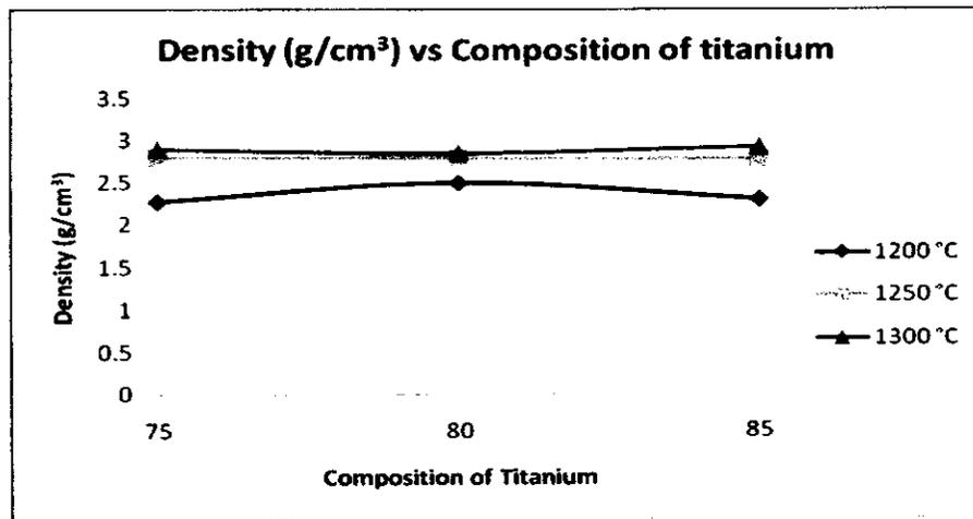
Figure 5: The effect of pure titanium content and sintering temperature on the density of the titanium foams
