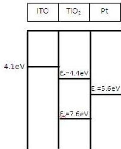
**Fig. 3** The band off-set of ITO/TiO<sub>2</sub>/Pt contact
