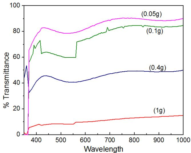
**Fig. 2** The transmittance spectra of TiO<sub>2</sub> thin films
