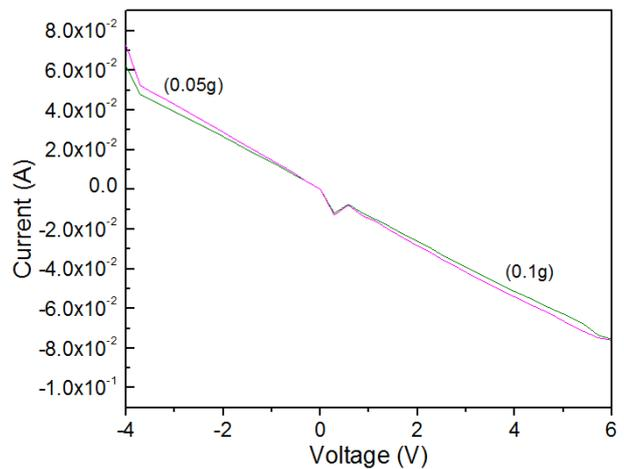
**Fig. 5** The Ohmic behavior of TiO<sub>2</sub> thin films
