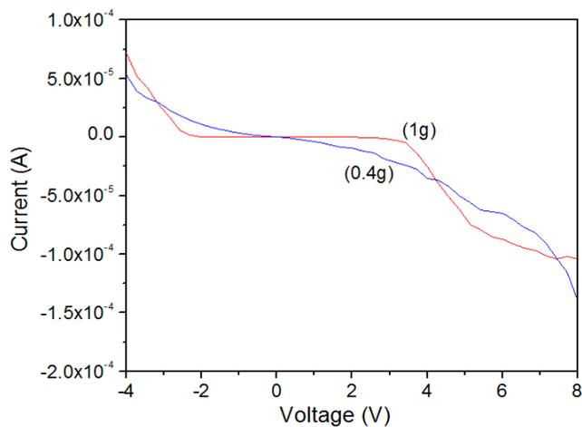
**Fig. 4** The Schottky behavior of TiO<sub>2</sub> thin films
