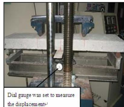
Figure 4: Four-points bending test setup
