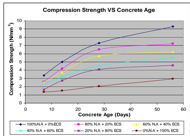
Figure 3: Compressive strength of pervious concrete
