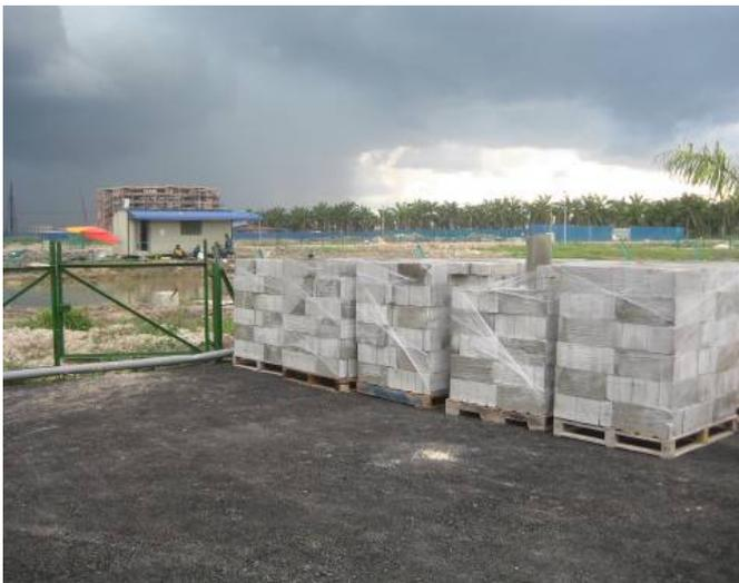
Photo 2: Biomass silica foamed concrete block for use as foamed aggregate
