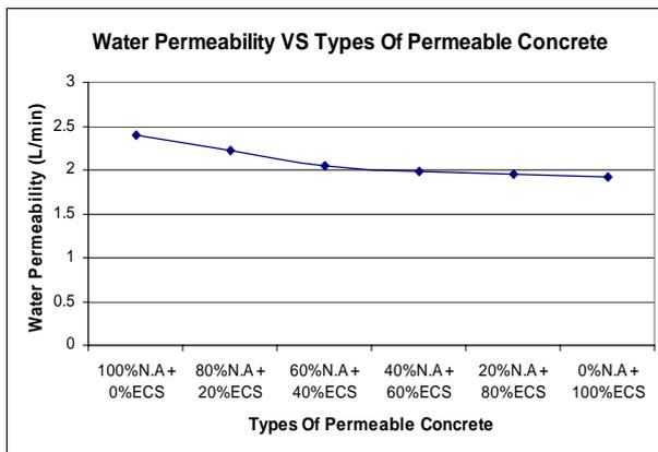
Figure 5: Water permeability of pervious concrete
