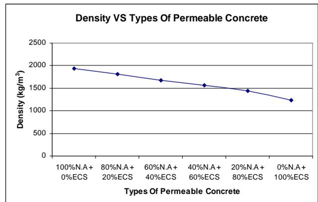
Figure 2: Density of pervious concrete
