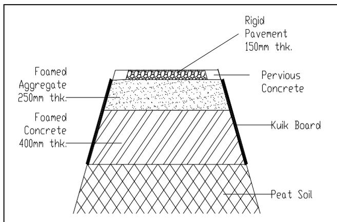
Figure 1: Typical cross section of road on peat
