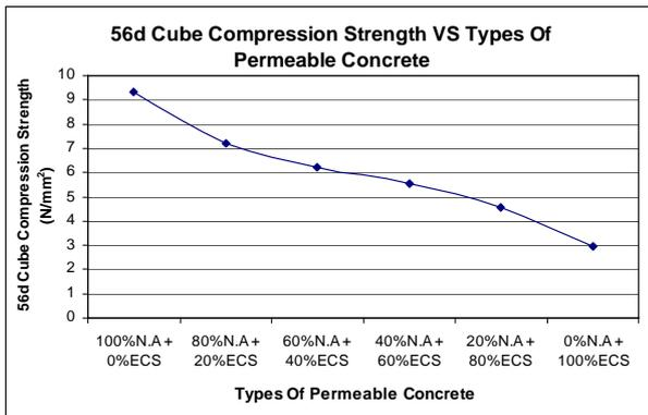
Figure 4: Compressive strength of pervious concrete at 56 days
