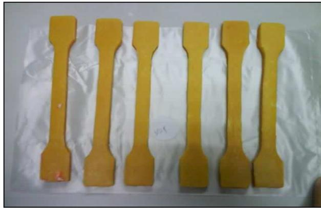
Fig. 1: Tensile test specimens of solid bio-polymer (VOP) fabricated by simple casting process
