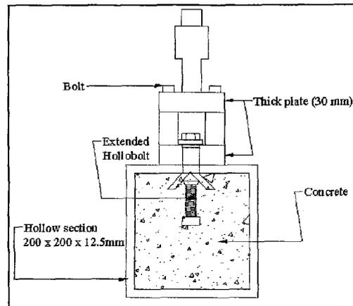
Fig. 3 Extended hollobolt in the concrete-filled hollow section
