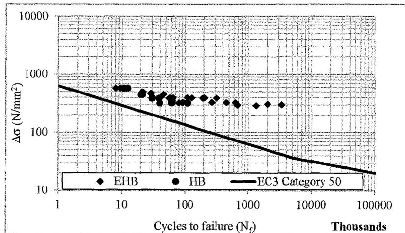
Fig. 5 Blind bolt comparison with classification of Eurocode 3
