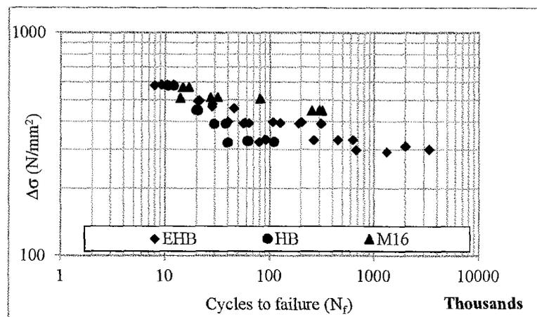
Fig. 4 Fatigue life of the blind bolt
