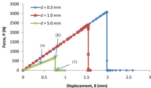
6 Typical load–displacement plots resulting from implementing XFEM approach for laminate reported by Kim et al.<sup>7</sup>
