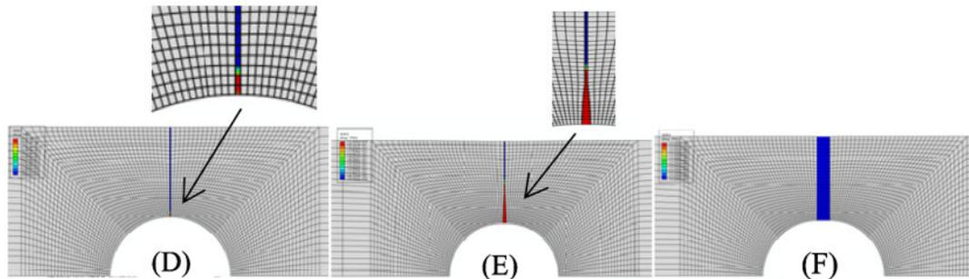
12 Damage plot for cohesive damage modelling using CZM as labelled in Fig. 9 for GFRP plate ( $d=10\text{ mm}$ ). Note that failure in cohesive zones is denoted as  $SDEG=1$  and given as red colour (D, E) and blue colour (F)
