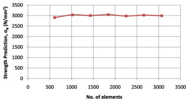
9 Notched specimen failure load as function of number of elements for woven glass–epoxy system (10 mm wide and hole diameter of 0.4 mm) following Kim et al.<sup>7</sup>
