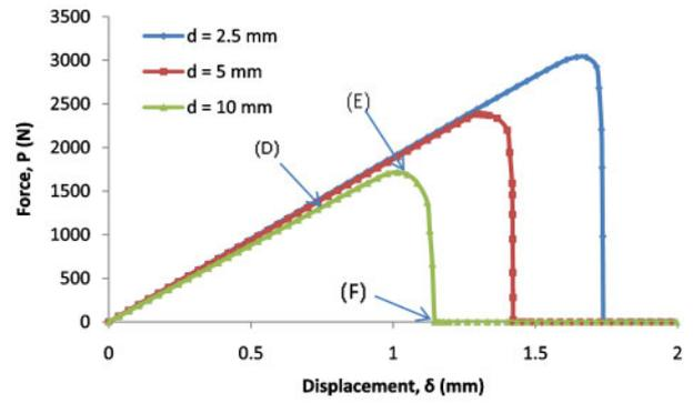
11 Typical load-displacement curve from CZM (woven GFRP (0°/90°/±45°)<sub>s</sub>)
