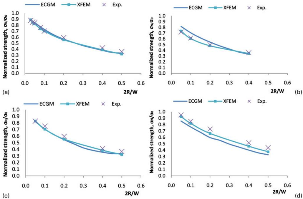
a glass-epoxy ( $W=10$  mm); b glass-polyester ( $W=30$  mm;  $v_{1f}=60\%$ ); c glass-polyester ( $W=30$  mm;  $v_{1f}=44.5\%$ ); d carbon-epoxy ( $W=10$  mm)
