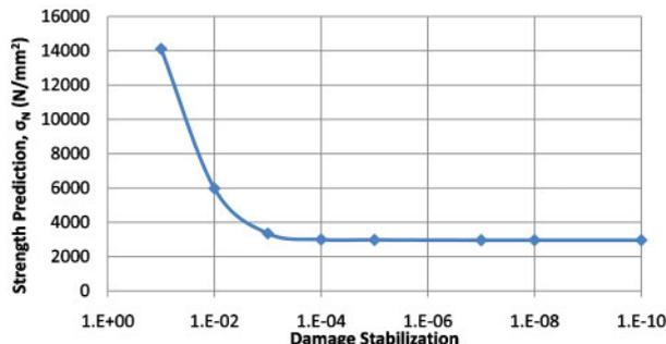
8 Notched specimen failure load as function of damage stabilisation coefficient for woven glass–epoxy system (10 mm wide and hole diameter of 0.4 mm) following Kim et al.<sup>7</sup>
