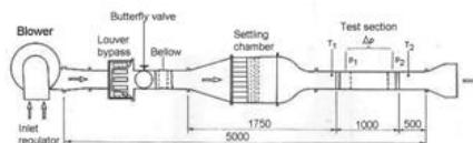
Fig. 1 Schematic diagram of the experimental set-up
