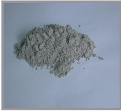
Fig. 2 Micronised Biomass Silica
