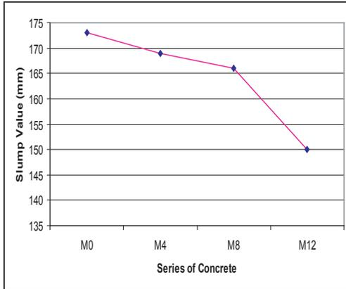
Fig. 3.1 Slump Value for MBS Concrete
