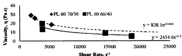
Figure 1: Viscosity (Expressed by power law model) vs. Shear rate for the feedstock F1 and F2 at T=140°C
