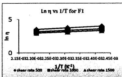
Figure 2: Vscosity versus Temperature for F1 and F3
