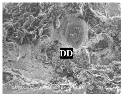
Fig. 5c Fracture Morphology of PWHT specimen in the weld metal region seen with Deep Dimples (DD)
