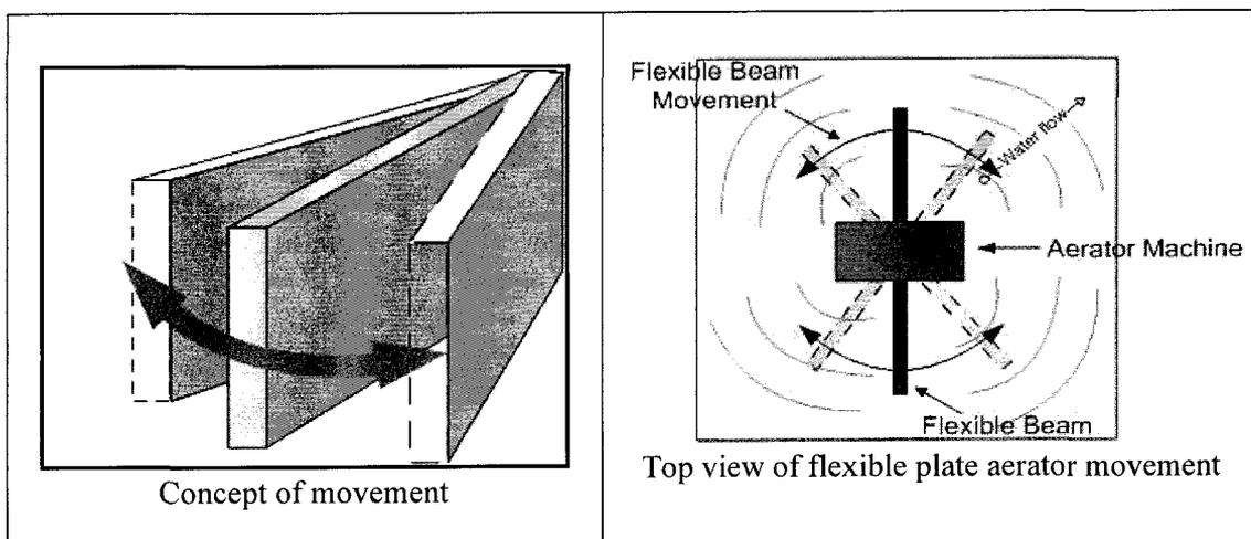
Fig. 3: Illustration of motion concept of the flexible plate aerator from top view
