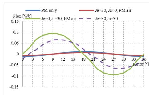
Fig. 6 Flux generated from PM, DC FEC and armature coil
