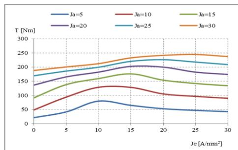
Fig. 8 Torque versus FEC current density at various armature current density
