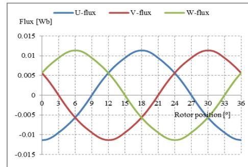
Fig. 2 Three-phase flux linkage produced by PM
