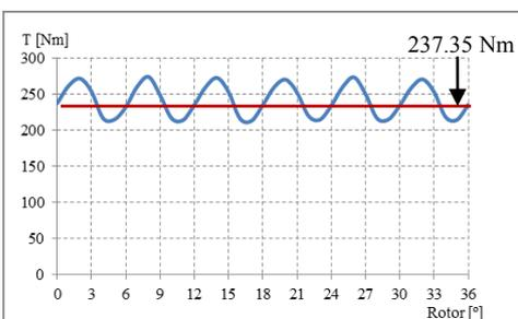
Fig. 7 Instantaneous torque characteristic
