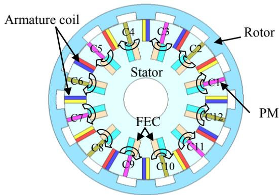
Fig. 1 Armature coil phase setting
