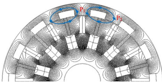
Fig. 3 Open circuit field distribution of the proposed motor
