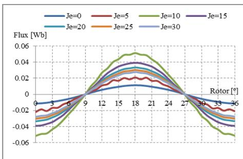
Fig. 5 Flux linkage at various DC FEC current densities
