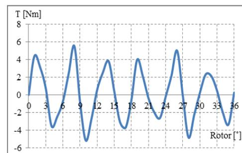
Fig. 4 Cogging torque of the proposed motor
