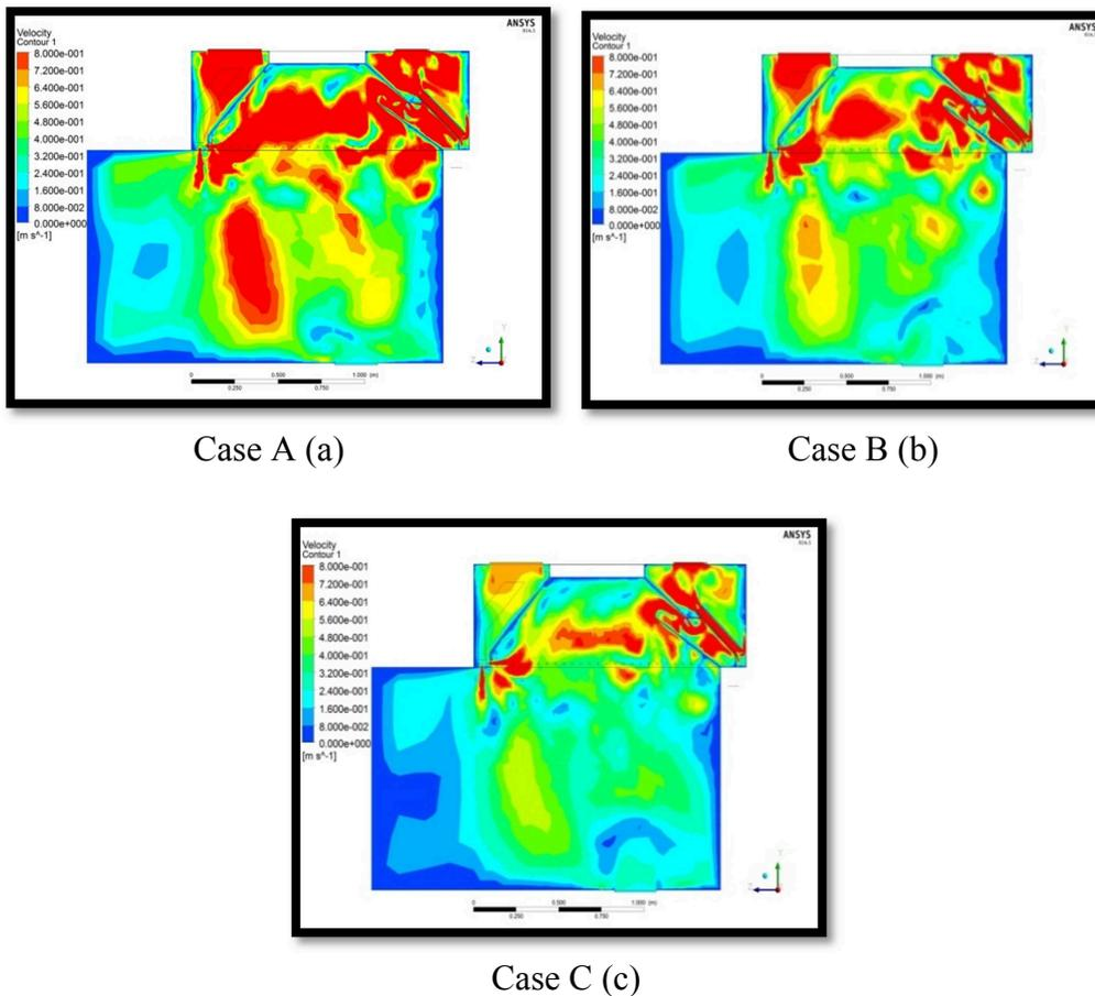
Fig 7: Velocity contour (m/s) for inlet capture jet with velocity for Case A (a), Case B (b) and Case C (c).
