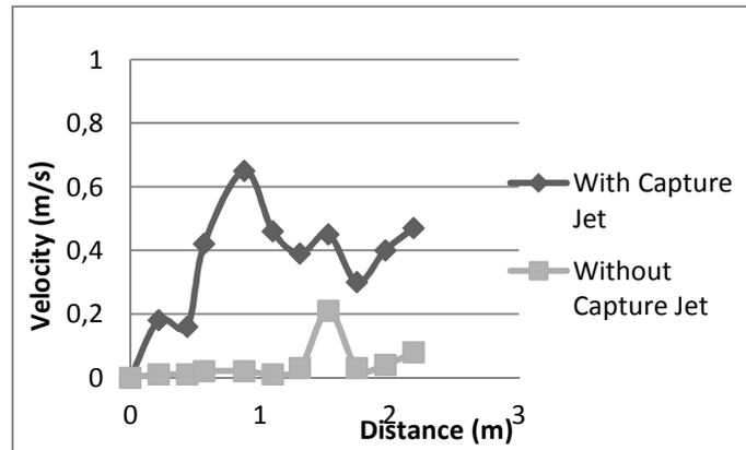
Fig 3: Graph of velocity (m/s) versus distance (m) for kitchen hood with and without capture jet technology at velocity inlet stove 0.235 m/s.
