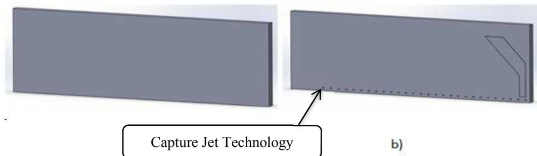
Fig 2: Side panel without capture jet (a) technology and with capture jet technology (b).
