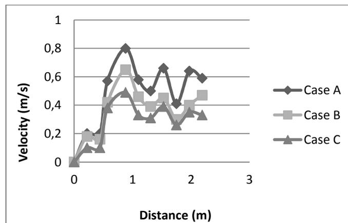
Fig 6: Graph of comparison of velocity (m/s) versus distance (m) for kitchen hood with capture jet between Case A, Case B and Case C.
