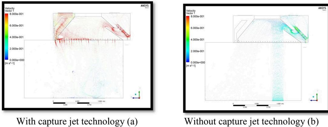
Fig 5: Velocity vector (m/s) for kitchen hood system with capture jet technology (a) and without capture jet technology (b) (yz-plane).
