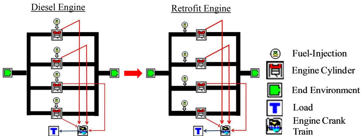
Fig. 1: GT-Power engine mapping computational model
