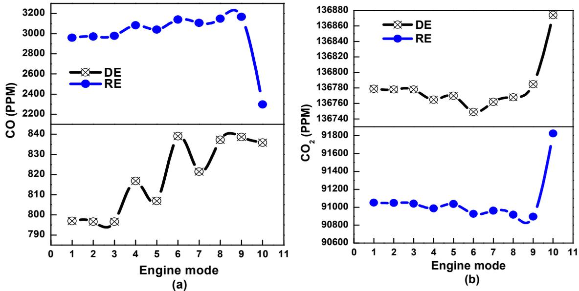
Fig. 4: CO and CO<sub>2</sub> emissions at engine mode condition
