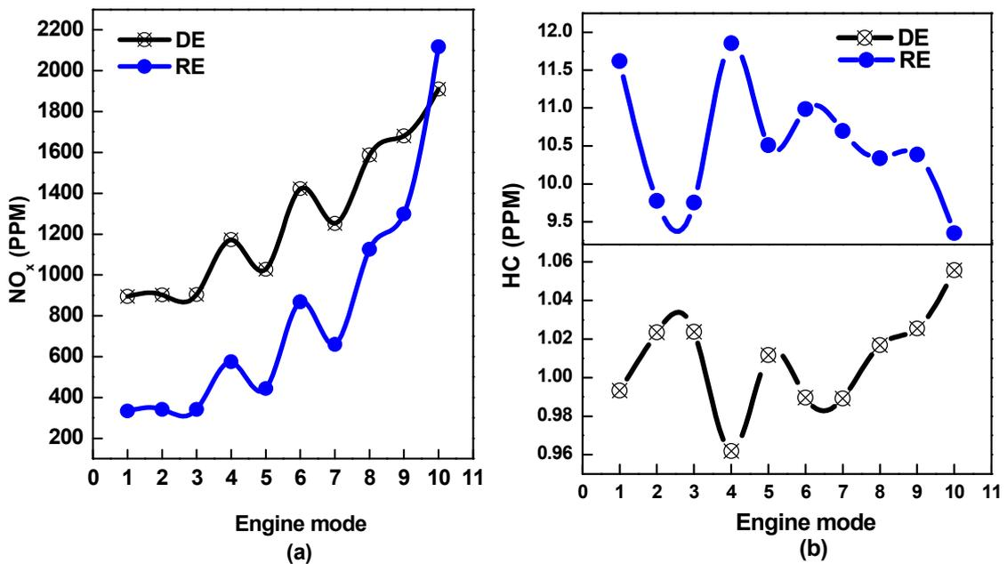
Fig. 3: NO<sub>x</sub> and HC emissions at engine mode condition
