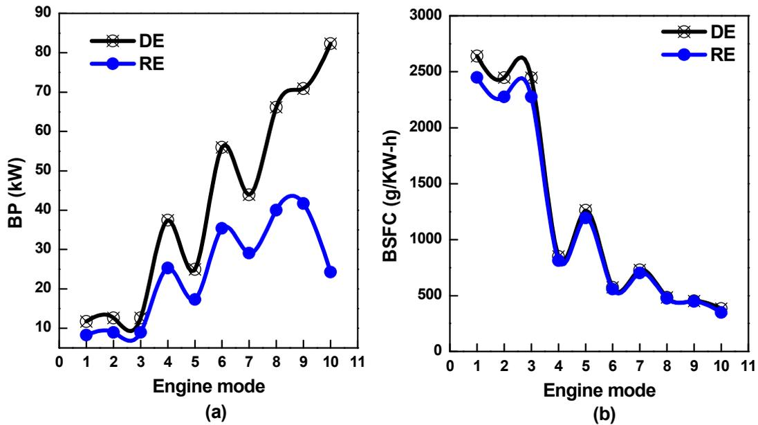
Fig. 2: BP and BSFC at engine mode condition
