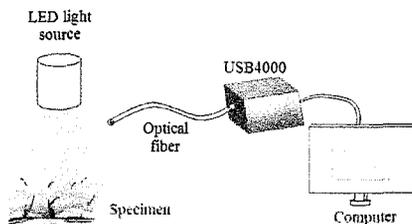
Fig. 1 Noncontact spectroscopy system.
