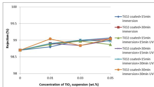
**Figure 4** Humic acid rejection with different of concentration of TiO<sub>2</sub> suspensions, immersion time and irradiation period
