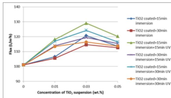
Figure 2 Pure water flux (PWF) with different of concentration of TiO<sub>2</sub>, immersion time and irradiation period
