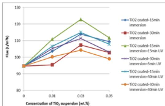
**Figure 3** Humic acid permeation with different of concentration of TiO<sub>2</sub> suspensions, immersion time and irradiation period
