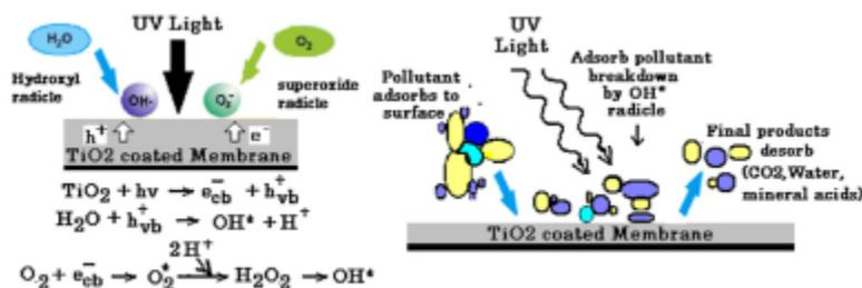
Figure 1 Photocatalytic mechanism and process
