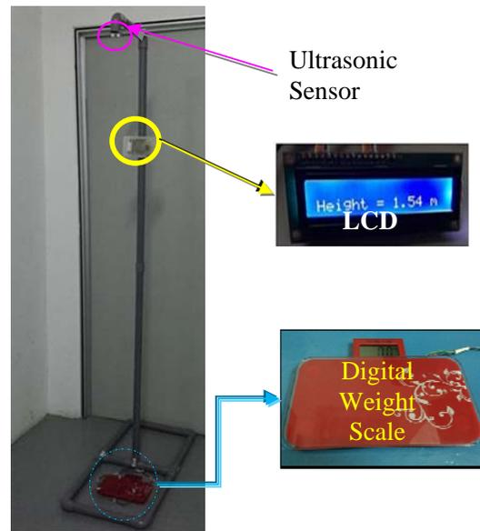
**Figure-2.** Prototype of measurement unit.
