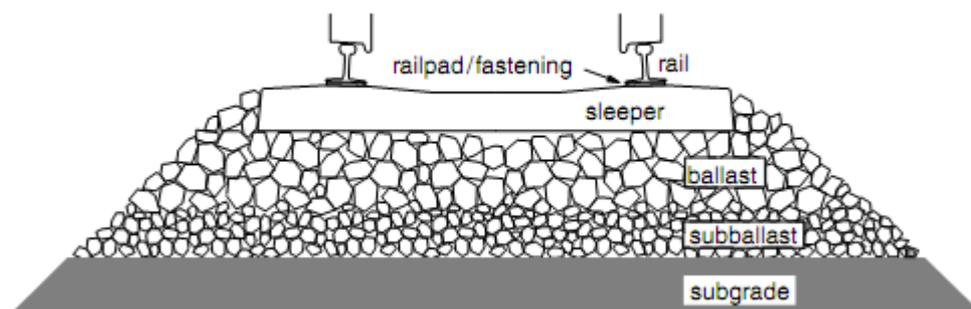
Figure 2.1: Components of track (Iwnicki & Dahlberg, 2006)
