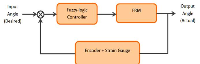
Fig.1. Block diagram of the system
