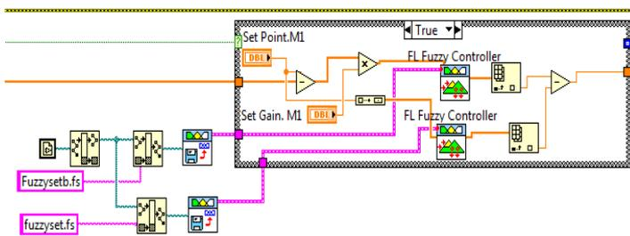
Fig. 8. LabVIEW block diagram of FLC system
